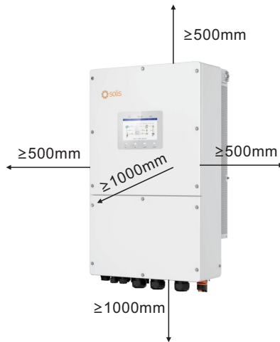
Figure 3.5 Inverter Mounting Clearances
